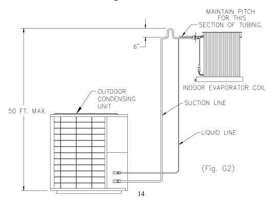
A gradual loop in the tubing can be constructed to take up the excess tubing if you find that too much tubing has been brought onto a job. Such a loop <u>MUST</u> be kept in a horizontal (flat) plane to avoid trapping the oil.
